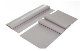
RH-PCM350Y It is a phase change material that has begun to soften at 45-55 °C. Compared with the traditional thermal conductive filling pad, the liquid filled pad can fill and cover the gaps and pits between the contact interfaces more effectively. On the other hand, it is in solid state at room temperature, providing convenience for assembly and use.
