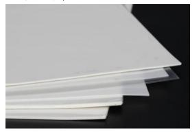
RH-PCM500Y It is a phase change material that has begun to soften at 45-55 °C. Compared with the traditional thermal conductive filling pad, the liquid filled pad can fill and cover the gaps and pits between the contact interfaces more effectively. On the other hand, it is in solid state at room temperature, providing convenience for assembly and use.
