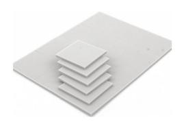
RH-GP400V thermal conductive silicon film is very soft and well compressed, which is used to fill the interface of two items, so that the air of the interface is discharged and the heat conduction efficiency is improved. The product has self-adhesive, can be die-cut into various shapes, easy to assemble. Thermal conductivity: W/M.K 4.0
