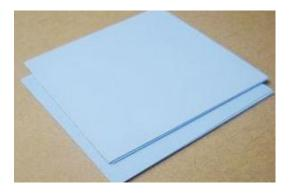
RH-GP350 thermal conductive silicon film is very soft and well compressed, which is used to fill the interface of two items, so that the air of the interface is discharged and the heat conduction efficiency is improved. The product has self-adhesive, can be die-cut into various shapes, easy to assemble. Thermal conductivity: 3.5W/m.k
