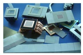
RH-PCM300 It is a phase change material that has begun to soften at 45-55 °C. Compared with the traditional thermal conductive filling pad, the liquid filled pad can fill and cover the gaps and pits between the contact interfaces more effectively. On the other hand, it is in solid state at room temperature, providing convenience for assembly and use.
