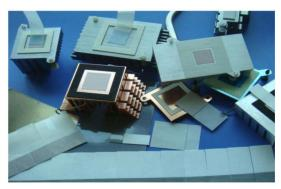
RH-PCM600 It is a phase change material that has begun to soften at 45-55 °C. Compared with the traditional thermal conductive filling pad, the liquid filled pad can fill and cover the gaps and pits between the contact interfaces more effectively. On the other hand, it is in solid state at room temperature, providing convenience for assembly and use.
